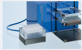
**Figure 2:** MACS® Elution Station and Elution Chamber enable positive and negative isolation.
