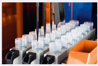
Figure 8: Cooled Chill Racks keep the samples and reagents at 2–8  $^{\circ}$ C.
