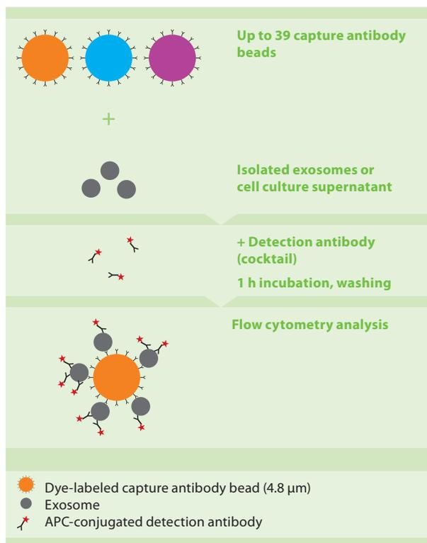
**Figure 2:** Principle of the MACSplex Exosome Kit.
